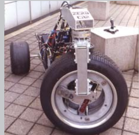
A prototype for the self-contained, digitally controlled Wheel Robot that can turn a full 360 degrees.
